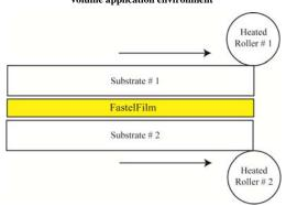
Apply heat using a hydraulic/mechanical press. Heat transfer through substrate # 1
