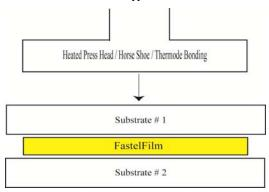
Clamp entire assembly together. Apply heat using multiple methods of heating including curing oven, heat tunnel or heat gun
