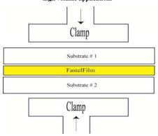
Process through top and bottom (or single) heated rollers. Heat will transfer through substrates.
