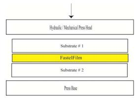
General setup for bonding and sealing heads of mechanical fasteners / plugs / screws. Apply heat using a curing oven, heat tunnel, heat gun, hydraulic or mechanical press.
